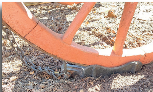
Drag shoe in situ. Wagon kindly supplied by the Richard Jefferies Museum, Swindon
